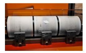
A seismogram is a recording of an earthquake's intensity. The greater the peaks on the graph, the greater the shaking - and the greater the shaking, the greater the earthquake's magnitude.
