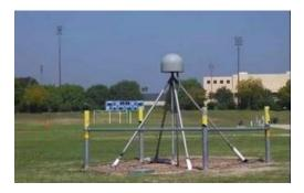
With GPS receivers like this one, scientists can use GPS data to measure tiny plate movements along fault lines. GPS also helps them measure plate movement after an earthquake.
